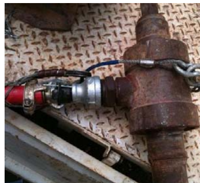
Correct method for attaching hose at rig end.
